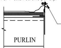
HAND CRIMP AT CLIP LOCATIONS AND FASTEN USING 2) 1/4-14 x 3/4" STITCH SCREWS PER CLIP
