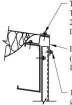
TEMPORARY 1/4-14 x 1 1/4" TEK SCREWS (556378) @ 24" (610) O/C TO SECURE INSULATION.
