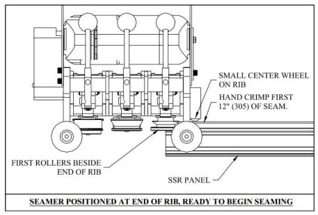
4. Switch the machine on and off until the rollers are all engaged and the seam is being formed properly.
