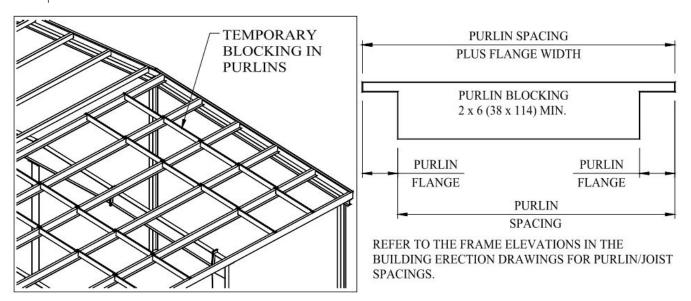
One **temporary** method of maintaining purlin alignment is to cut and install 1 1/2" (38) thick blocks as shown. The blocks should be as wide as possible (5 1/2" (114) minimum). At least one row of blocking in a bay should be used. Use additional rows as required. **This temporary blocking must be replaced by permanent purlin stabilizers as roofing progresses.**
