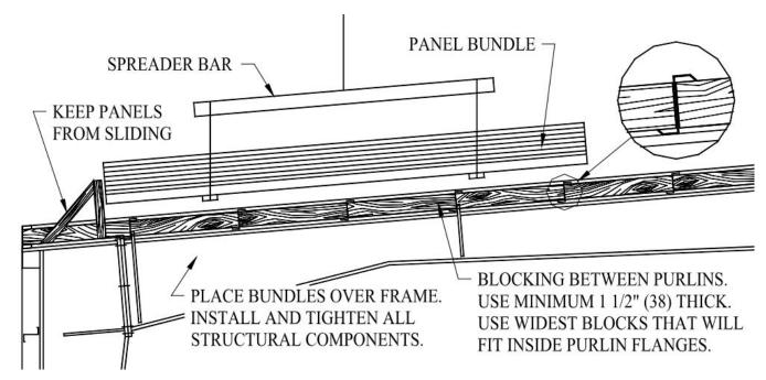
**Carefully consider the arrangement of the bundles on the roof.** Determine how much roof will be covered by each bundle and space them accordingly. Orient the bundles the same way they will be installed (refer to "PREPARATION: START POINT AND DIRECTION OF INSTALLATION"). Avoid placing bundles where they will interfere with string lines, traffic, equipment, etc.
